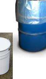
**Plastic Combi Drums** are a new drum type that have only become available recently. Like their steel counterparts they are open top drums that are approved to carry both liquids and solids. The one pictured on the right has a bung in the centre for filling with liquid like tight-heads. For now they are only available a 150 litre size but other sizes should become available in the future.
